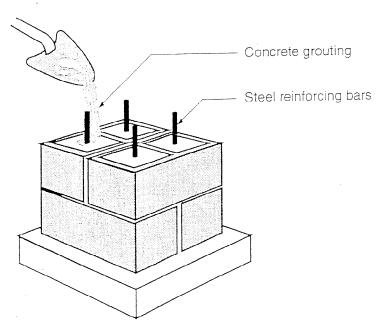
For piers exceeding 80 inches in height, the concrete blocks should be filled with concrete grouting and steel reinforcing bars should be utilized.
