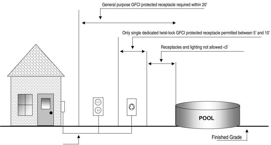
Branch circuit for permanent pools (those capable of being filled with over 42" of water) shall be pulled in electrical non-metallic tubing (PVC). Burial depth shall be a minimum of 18". Receptacles shall GFCI protected.
