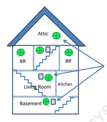
Smoke detectors are required on each level of a dwelling unit (NOT including crawl spaces or uninhabitable attics)
