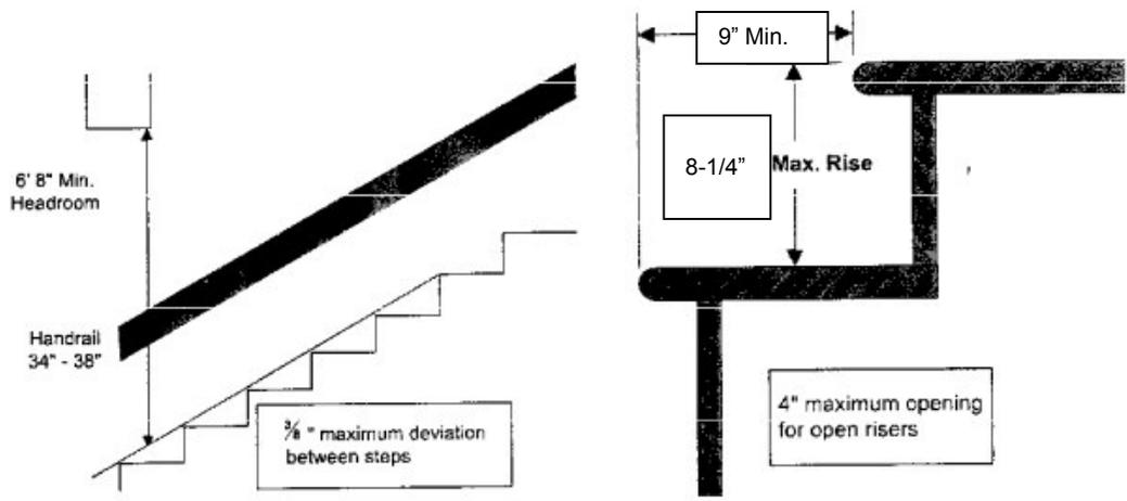
**Figure 3.14: Stair Geometry**
