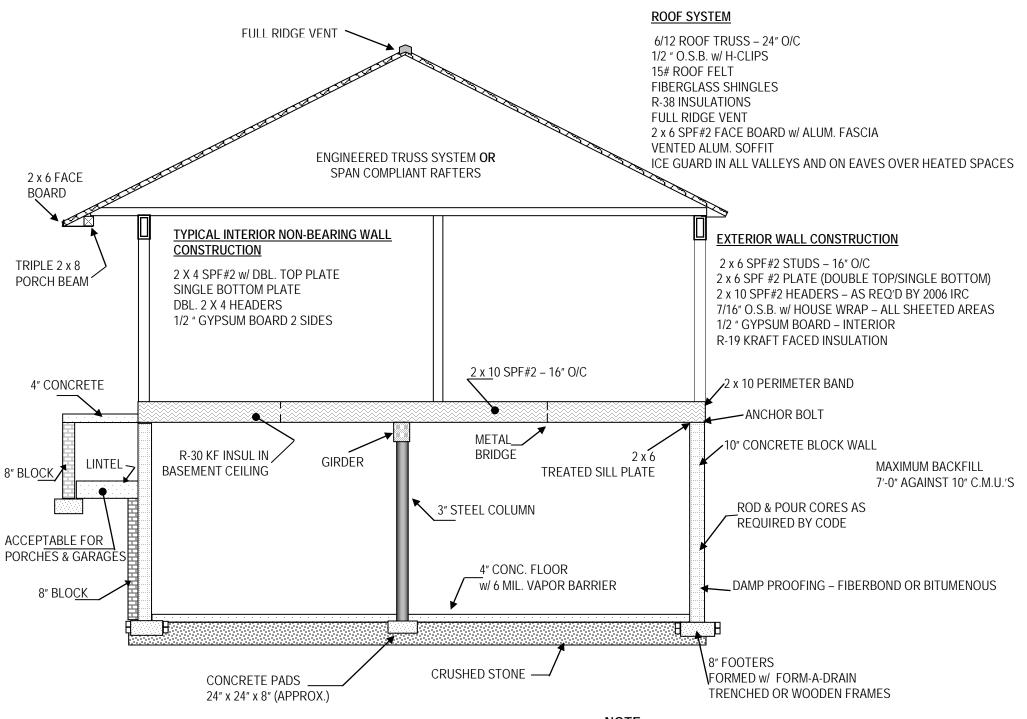
**NOTE:**TYPICAL DETAIL FOR CONSTRUCTION STANDARDS
